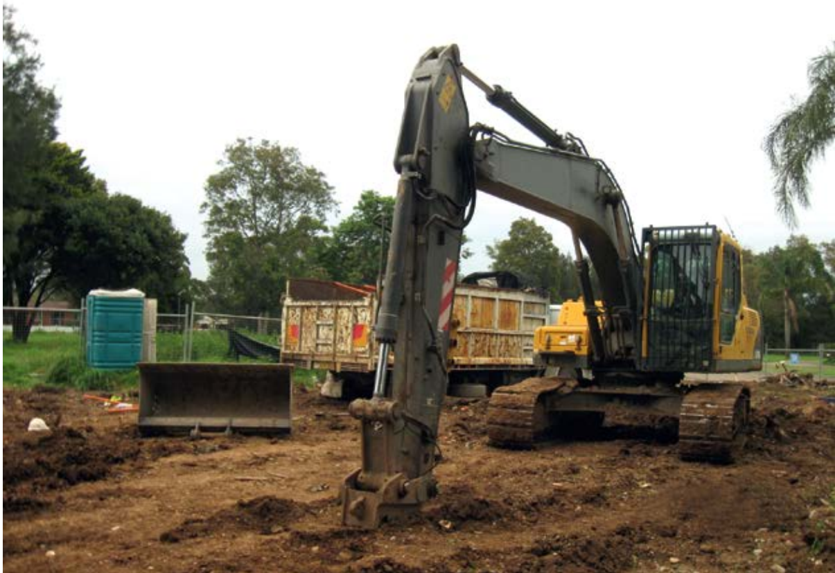
Photo 1: The deceased was positioned next to the truck trailer when struck by the bucket.
