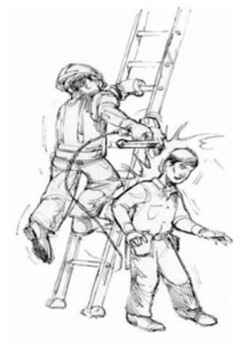
Figure 2: This image depicts an inadvertent discharge whilst ascending or descending a ladder.
